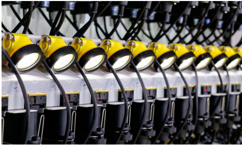
Example of charging rack LC-1/51 - equipped with three load banks; enables simultaneous loading of 51 lamps. Charging for 68, 85 or 102 lamps have 4, 5 or 6 load banks respectively.
